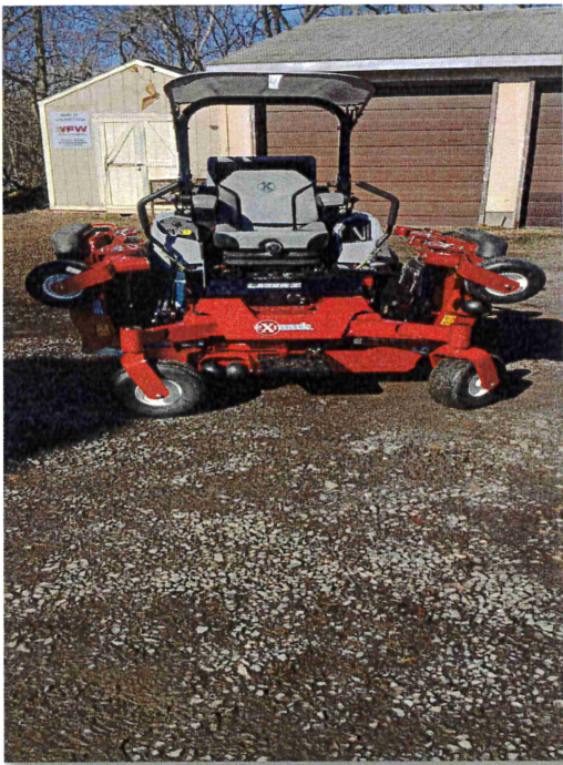
Wings up for Transport Mode
