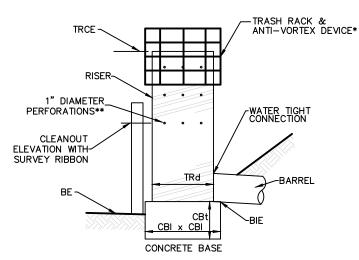
\* SEE STANDARD CONSTRUCTION DETAIL #7-5, TRASH RACK AND ANTI-VORTEX DEVICE \*\* LOWEST ROW OF HOLES AT SEDIMENT CLEAN-OUT ELEVATION
