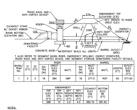
SEDIMENT BASINS, INCLUDING ALL APPURTENANT WORKS, SHALL BE CONSTRUCTED TO THE DETAIL AND DIMENSIONS SHOWN ON THE E&S PLAN DRAWINGS.
