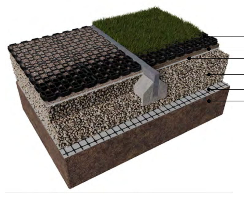
GRASSPAVE2 - TYPICAL CROSS SECTION (BASIN MAINTENANCE ACCESS PATH) (NOT TO SCALE)
