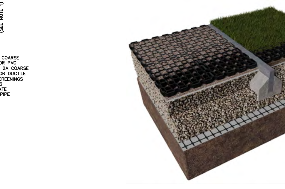
GRASSPAVE2 - TYPICAL CROSS SECTION (BASIN MAINTENANCE ACCESS PATH) (NOT TO SCALE)
