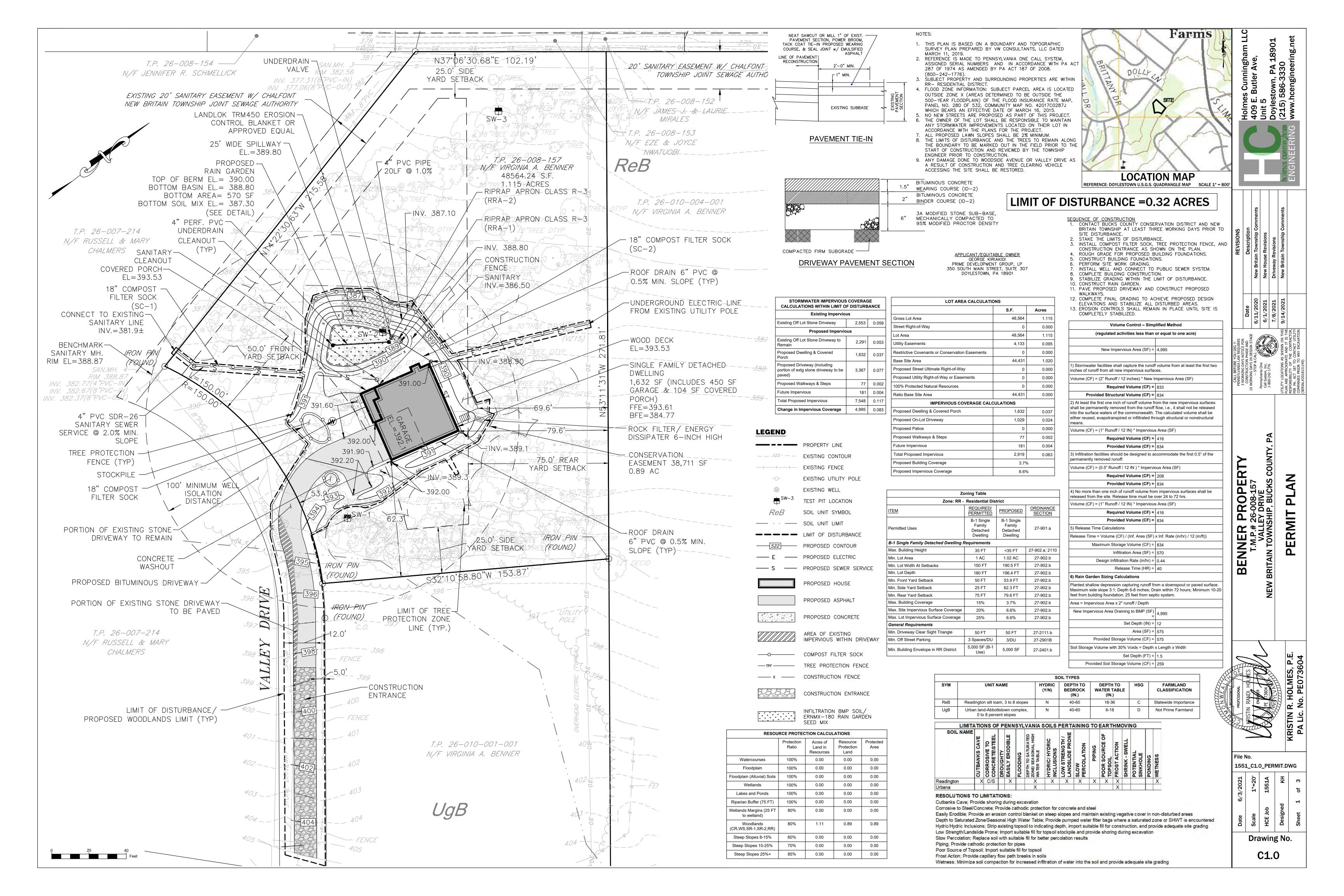
STOCKPILE HEIGHTS MUST NOT EXCEED 35 FEET; STOCKPILE SLOPES MUST NOT EXCEED 2L:1V.
